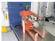
Figure 1 Thorax Certification of a Crash Test Dummy
